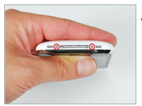
Remove the two 3.7mm Phillips #00 screws from the dock-connector end of the iPhone.
