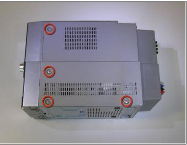
Using a Phillips screwdriver, remove the eight 9.5 mm screws on the left and right sides of the device.
