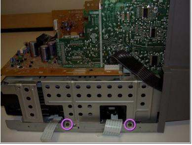
Using a philips screwdriver, remove the four 9.5 mm screws indicated and place aside.
