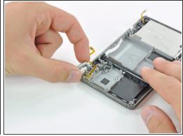
Press lightly on the back of the button until it becomes unattached. Be careful not to lose the small spring and pin behind the plastic button.
