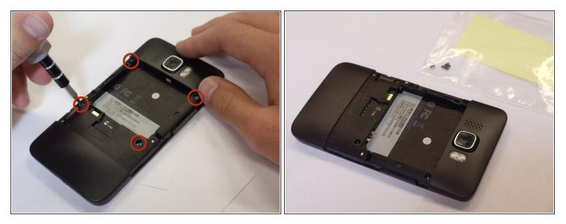
• Remove the four black 3.5mm T5 screws from the back of the phone.
