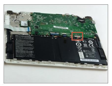
Pull the battery connector cable towards the battery to disconnect it.
