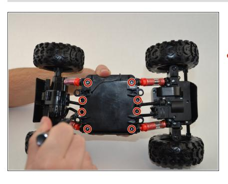
Use the Driver and bit J1 to remove the top under-body plate by unscrewing the eight 9.5mm Philips screws.
