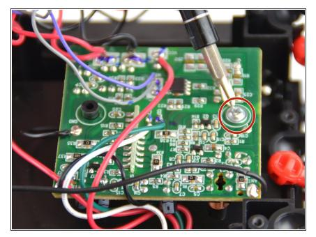
Use the driver and bit J1 and remove the 7.7mm Philips screw highlighted.
