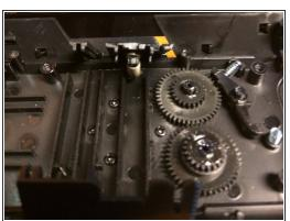
Now your should be left with this bottom part. To get to the sprockets and the locking mechanism inside, you need to remove the plate that is secured with 4 screws + 1 smaller screw. When that plate is removed (might take some slight convincing) you will see the sprockets and mechanism seen in picture 2 and 3.
