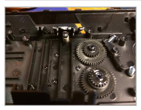
• Mind the small spring in picture 1 when assembling, this pulls both the clamps out when the button is pushed. Also remember to realign all the parts when assembling. Other than that it is the reverse of dissasembling.
