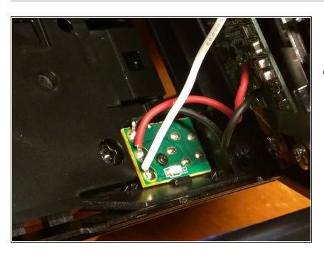
Next you need to be careful not to brake any of the 3 wires running from the main charging circuit to the power intake port, that sits on a seperate chip in the bottom housing. This is held on by 1 screw.
