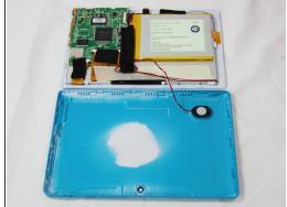
• Use the plastic opening tool to pry the back off the tablet. Work your way around the edges. Once you have one side open you can slowly unsnap the rest of the case and use the tool as needed.
