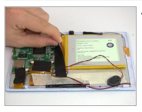
Pull back the tape to expose the wires that are attached to the battery.
