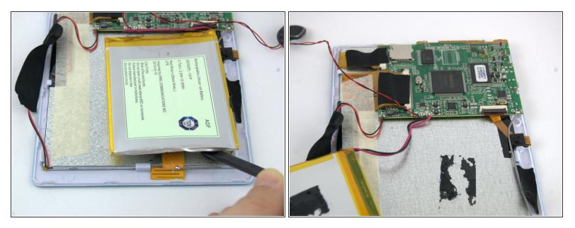
A Do not attempt to fully remove the battery. It is still connected to the motherboard by two wires.
