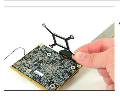
Remove the clamping bracket from the back of the GPU.
