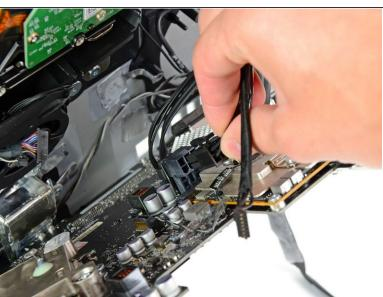
Depress the locking mechanism and carefully pull the DC-In cable out of its socket on the back of the logic board.
