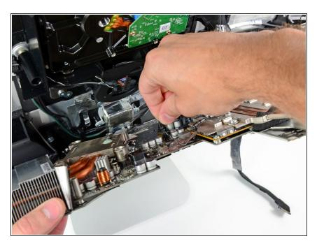
Disconnect the LCD temperature cable by pulling its connector up and out of its socket on the logic board.
