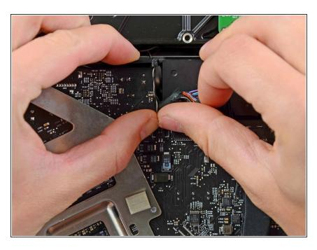
Use your thumbnails to push the right temperature sensor connector toward the top edge of the iMac and out of its socket.
