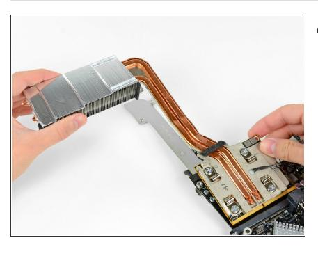
Lift the GPU heat sink slightly and pull the GPU board out of its socket on the logic board.
