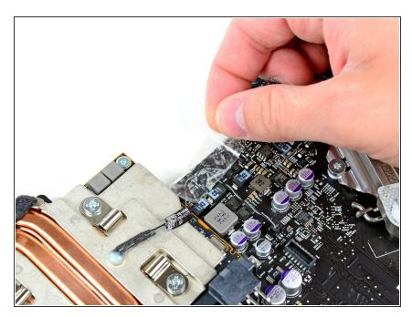
Remove the strip of tape securing the GPU thermal sensor cable to the logic board.
