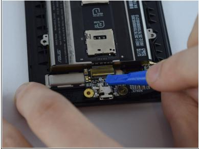
Using the plastic opening tool, unlock the ribbon cable indicated in the picture by prying up the yellow tab.
