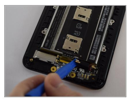
Using a plastic opening tool, remove the vibration motor from its housing.
