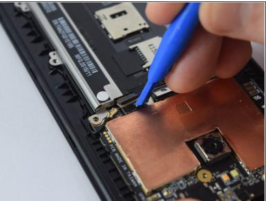
Using the plastic opening tool, gently pry the ribbon cables up as indicated in the pictures.
