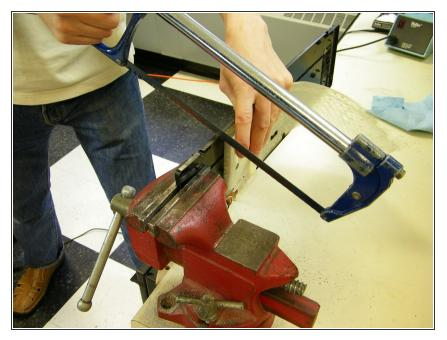
• Cut the bottom part of the keyboard too. Fold or remove the plastic PCB out of the way when cutting.
