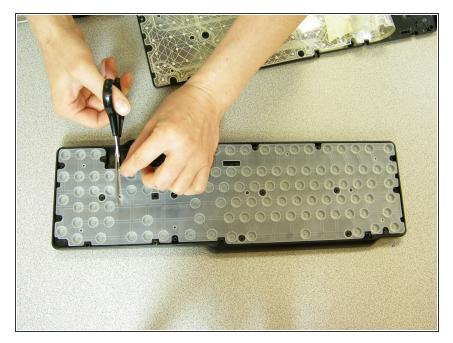
• Take the keyboard apart. You will find a white rubber sheet under the top part of the keyboard. Cut off the part for the numerical keypad.
