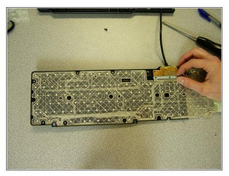
• Screw the PCB and the metal bar back on.
