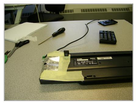
Since you have cut the portion of the keyboard with the supporting leg for tilting, supply it with a new leg. You can use a key from the numerical keypad.
