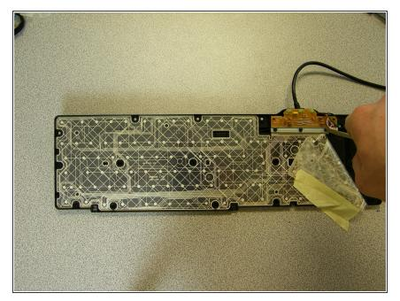
• On the bottom part of the keyboard, remove the three screws and the metal bar holding the keyboard PCB and fold the plastic sheet so it is out of your way when cutting.
