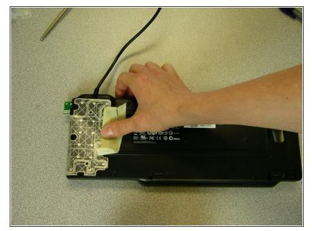
Assemble the rest of the keyboard, and fold the plastic sheet under your keyboard. Do not cut it because it will render the keyboard useless.
