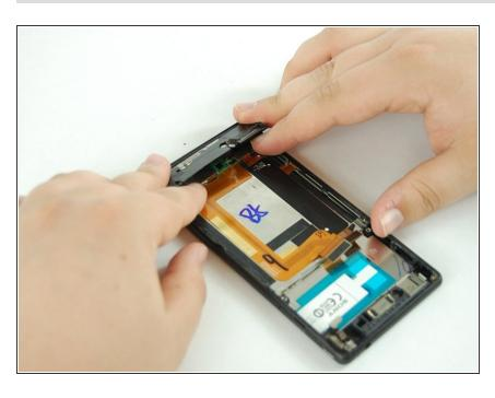
Remove the Metal LCD assembly cover by lifting up and pulling it out away from the edge of the phone, towards the middle. Disconnect the LCD connector. The assembly cover is flexible and can be bent, be careful when applying force. Carefully unstick the connector from underneath the LCD cover
