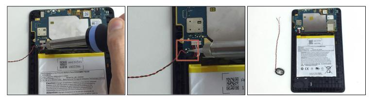
• Desolder the speaker wires from the motherboard.
