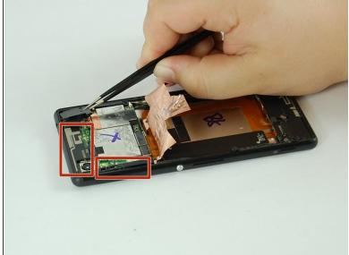
Remove three pieces of the securing bracket using tweezers
