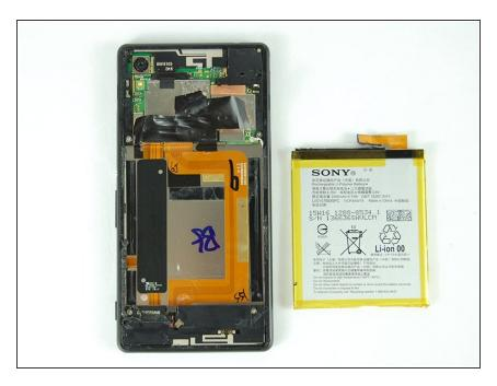
Remove the battery once all of the adhesive is broken, and the connector is unplugged.
