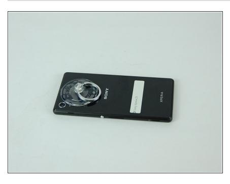
Attach a suction cup to the back of the M4 Aqua by carefully pushing down on it near the top of the phone.
