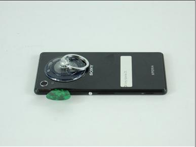
While Pulling on the suction cup, slide a thin plastic spacer (guitar picks work well) between the back cover and the phone. Slide it around the edges to break the adhesive seal. Be careful, but don't be afraid to use some force. You should hear a sticky breaking sound.
