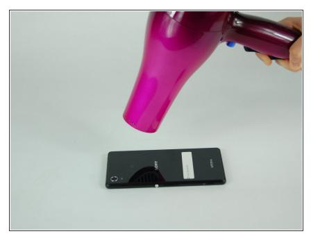
Place the phone face-down, and use a heat gun or hair dryer to evenly heat the back surface until to soften the adhesive.
