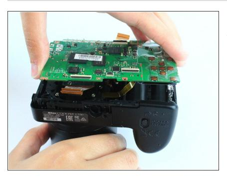
Remove the motherboard by lifting it directly up. To reassemble your device, follow these instructions in reverse order.
