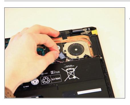
Once the bottom cover is removed, peel away the piece of tape located near the fan and heat sink assembly.
