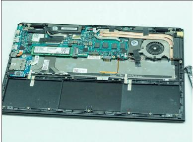
Finally, remove the track pad from the computer.
