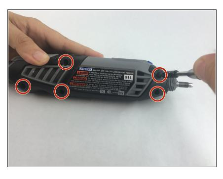
Using the Torx 15 screwdriver tip, remove the 5 screws (12.5 mm) that hold the casing together.
