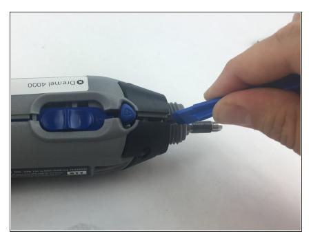
Use a plastic opening tool to gently wedge apart the hard plastic threads.
