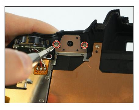
Remove 2 screws from back of EVF/LCD button.
