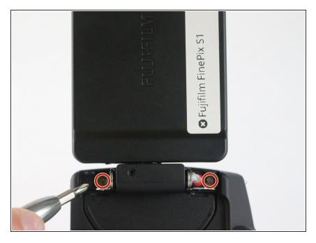
Remove the 2 screws from under the LCD hinge caps.
