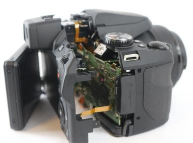
Carefully pull the back body off of the camera.
