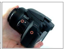
Remove the 7 screws on the perimeter of the camera body.
