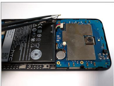
Using tweezers, disconnect the antenna wire.
