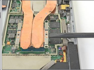
• Use the flat end of a spudger to gently pry the heat sink straight up and off of the CPU.
