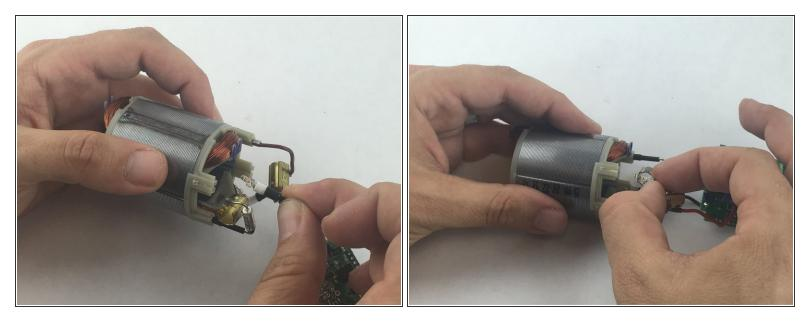
• Firmly hold the field assembly in one hand, and carefully pull free the red and black wires that connects the electrical assembly to the field assembly.
