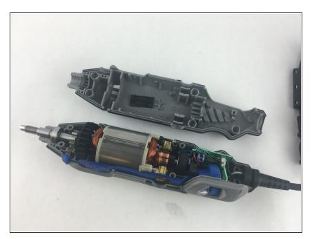
• Use your hands to carefully remove the back casing so that none of the components fall out.
