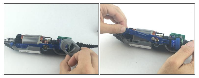
To clear access to the electrical assembly, remove the variable speed dial cap and blue power lever, and set them aside.
