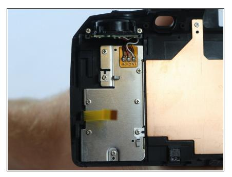
Remove all 10 screws from the metal fitting inside the back of the camera.
