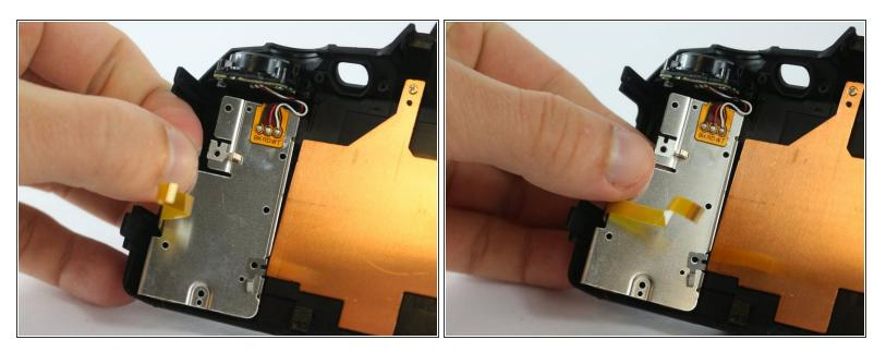
• Lift up on the metal fitting and pull it out of the camera.
