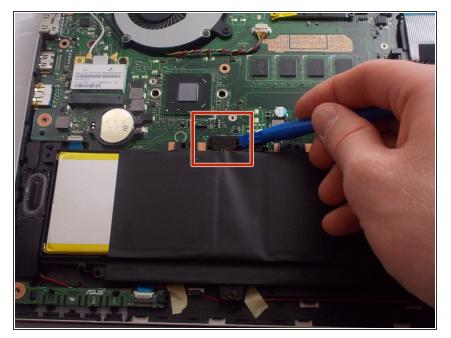
Disconnect the one flat topped wire connector by carefully using a plastic opening tool to pry up both sides and then lifting the connector from its socket.
