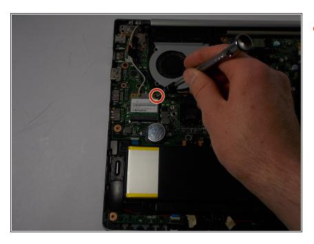
Remove the one 3 mm Phillips head screw holding the Wi-Fi card in place.
