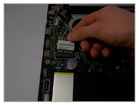
• Carefully slide the card out of its connection port by pulling it outward.
