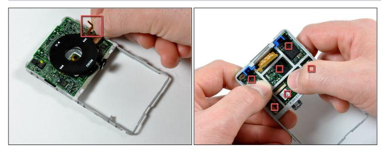
• Turn the iPod over and peel the orange click wheel ground tab up from the metal framework.
