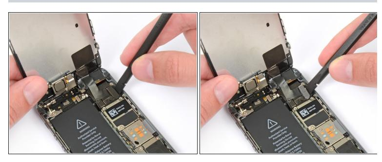
• Use a spudger or a fingernail to disconnect the front-facing camera and sensor cable.
