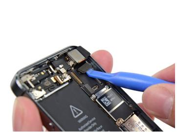
Using a plastic opening tool, disconnect the rear-facing camera cable connector from the logic board.
