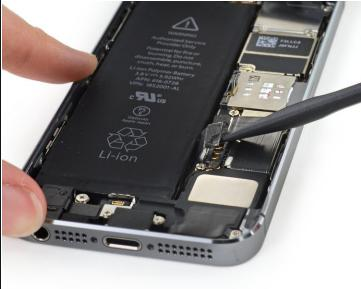
Use the flat end of a spudger to gently pry the battery connector up from its socket on the logic board.
