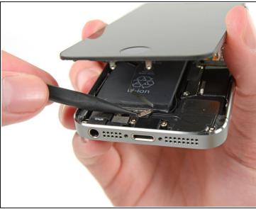
• Use the tip of a spudger to pry the home button cable connector up out of its socket.
