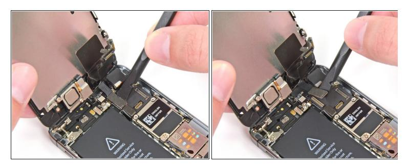
• Finally, disconnect the digitizer cable connector.
