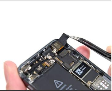
• Using a pair of tweezers, flip the rubber camera cover out of its clip, and toward the outside of the rear case.
