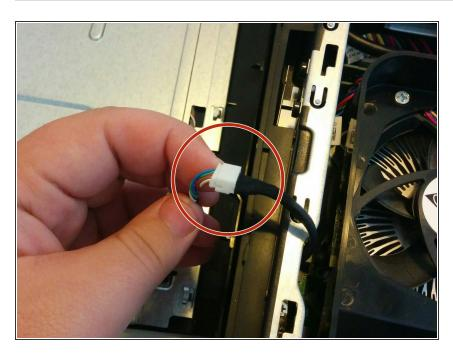
Lift the side panel off, and gently flip it over the top of the system, being careful not to break the LED control cable. Unplug its connector and set the case panel to the side.
