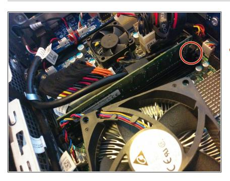
Now, push the white latch (circled in red) DOWN and pull the ram card straight up to a ~45 degree angle.
