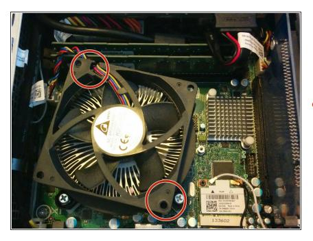
Next, remove the screws securing the plastic air re-director (not shown in picture) to the fan, and gently lift it
