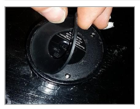
• You can pick at the edge of it and carefully peel it off. There's a piece of double-sided tape in between it and the plastic base that may remain. If you're careful you can peel it off intact and reattach it to the rubber foot. This step exposes the screws that hold the circuit board to the speaker.
