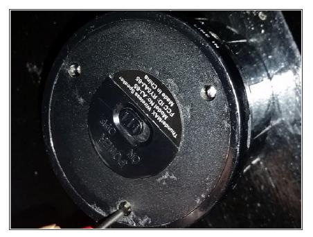
Using a small phillips head or even a small enough flat head, remove the three screws. Then you just pull a bit on the bottom, underneath the crease that goes all the way around the cylinder. It's the crease that contains the volume knob, control buttons, input jack, etc
