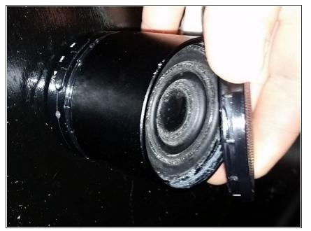
With a little coaxing, the top ring with the speaker screen pops off. If you've been using this speaker long enough to need to take it apart, chances are this piece has popped off before on accident.
