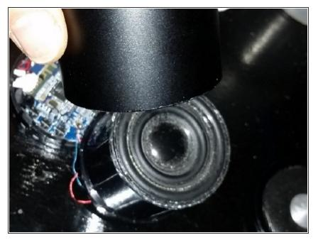
• This is how the metal outer cylinder looks after you pull it off the inner cylinder that holds the speaker.
