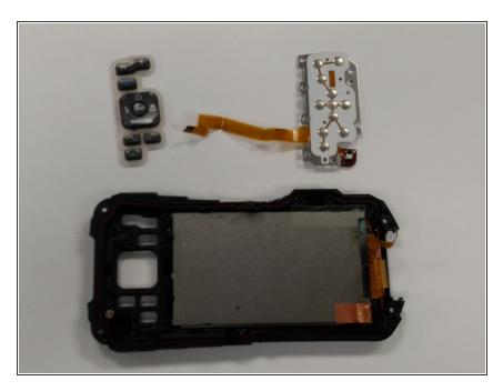
• Once panel is removed the button 'sheet' can be removed.
