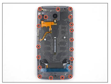
• Use a T3 Torx driver to remove twenty 2.4 mm screws.
