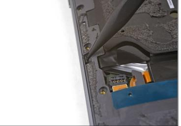
• Use the point of a spudger to push the small clip securing the left side of the midframe toward the edge of the phone, releasing the clip.
