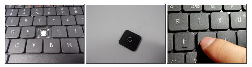
(i) Before placing, check that the key is properly orientated. The letter side should be face up.
