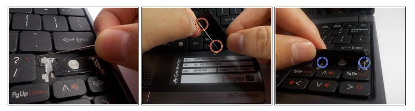
A Option two is to be used if the key cannot be attached without removing the metal bar.
