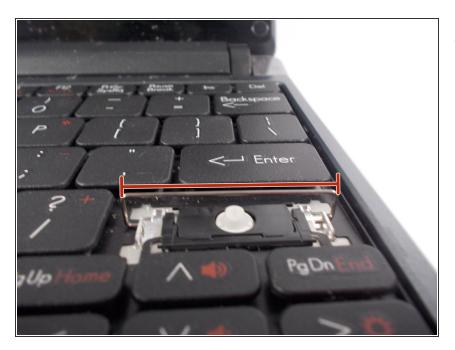
Large rectangular keys need to be attached to the small metal bar to be attached properly. There are two ways to do this.
