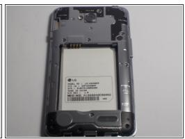
Remove the eleven 4mm screws using a Philips head screw driver.
