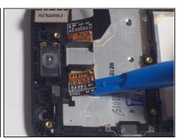
Using the blue lifting tool carefully remove the screens connectors.
