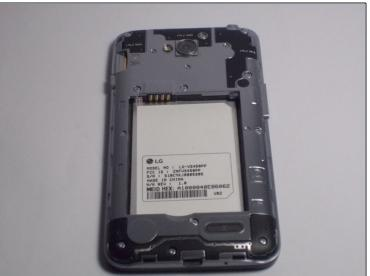
Flip the device over and remove the back covering.
