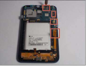
Disconnect the remaining ribbon plugs and connectors. (Only remove the highlighted cables for the removal of the logic board.)
