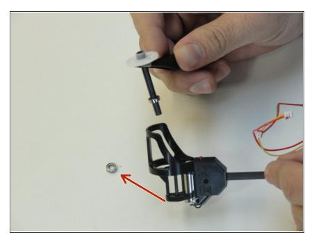
Once the ball-bearing is removed, use tweezers and remove the entire tube and gear from the drone arm assembly.
