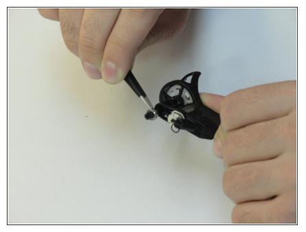
• Use a pair of tweezers to remove the silver nut from the bottom of the carbon tube.
