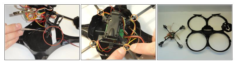
• If present, remove the white tape over the black and red wires on the head lamp with a spudger.
