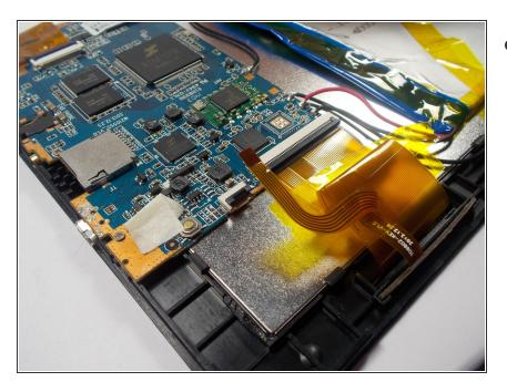
Then remove the ribbon cable from the ZIF connector.
