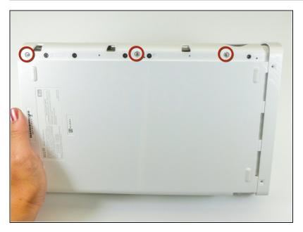
On the bottom of the console beneath the previously removed faceplate, remove the three 13.2mm Tri-wing Y1 screws.
