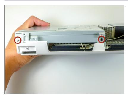
On each side of the DVD drive, remove the two 4.6mm Phillips #0 mounting screws.
