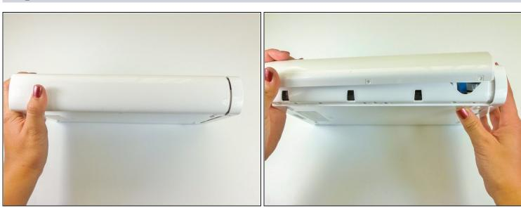
• On the side opposite of the exhaust vents, slide the cover faceplate towards the back of the console and pull upwards to release it.
