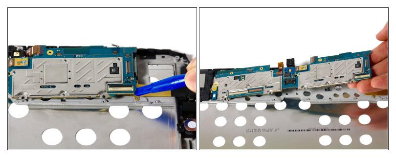
• Remove motherboard by gently pulling upward under its corner.
