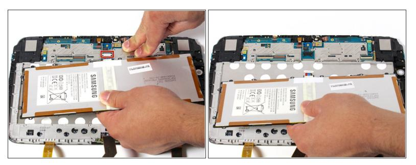
Disconnect the battery by lifting it upward and pulling it away from the connector.
