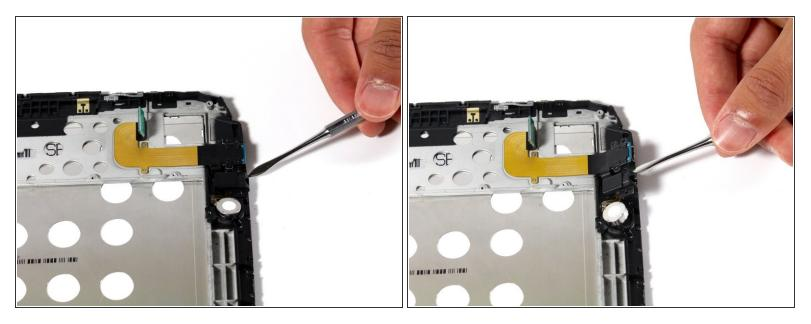
• Lift the assembly by gently applying upward pressure with the spudger on the assembly.
