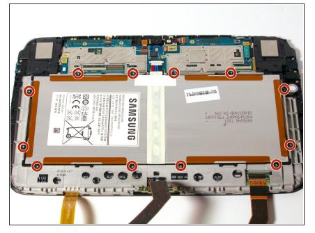
Remove the twelve 2mm screws around the perimeter of the battery with a PH00 screwdriver.
