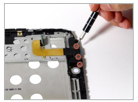
Remove the three 2mm screws along the right side of the device using a PH00 screwdriver.
