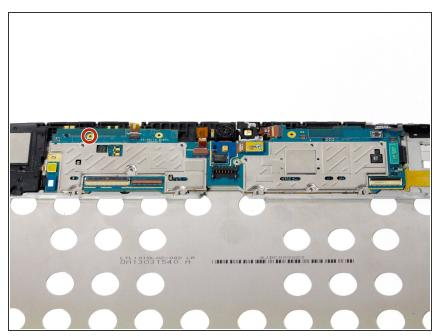
• Remove one screw on the logic board with a PH00 screwdriver.
