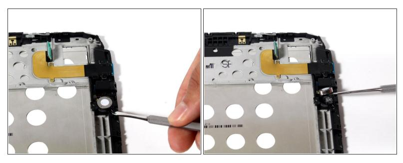
• Unseat the small vibrator motor by gently applying upward pressure with a spudger.
