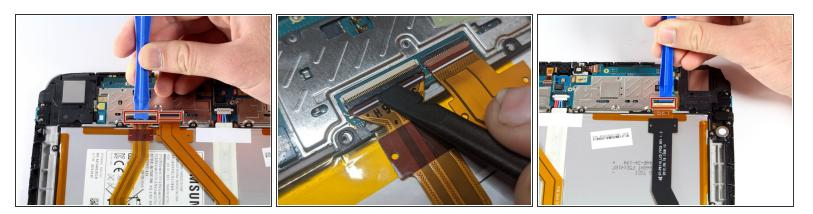
• Detach the three connector ribbons passing over the battery using the plastic opening tool.
