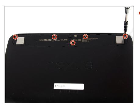
Remove the five 2mm screws on the back of the device using a PH00 screwdriver.
