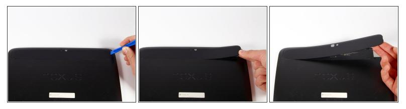
Using a plastic opening tool, remove the thin plastic cover from back of the tablet by prying up from its small tab.
