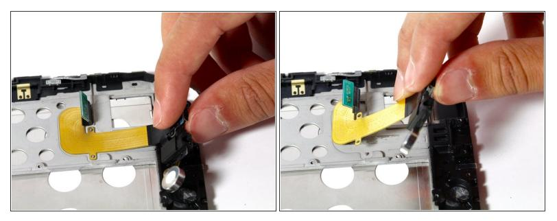
Gently pull battery-audio jack-USB assembly upward, detaching it from its adhesive.
