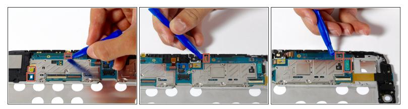
• Disconnect connectors around the perimeter of the motherboard.
