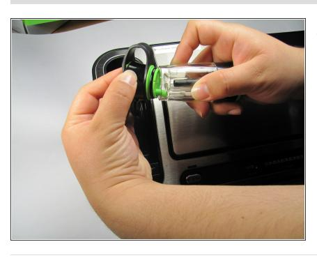
Pull the black top (identified with the rubber loop) from the liquid chamber. You may now replace/clean the accessory.
