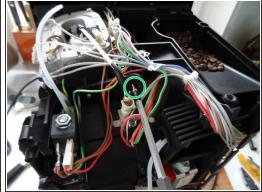
The boiler and valve are fixed with three screws. Also loosen some cables and hoses until the boiler can be removed.
