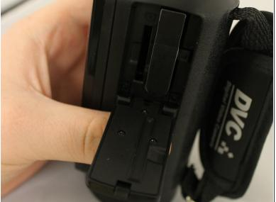
Pull back the tab to reveal the battery compartment.
