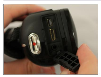
• Open the cover to reveal the device ports.
