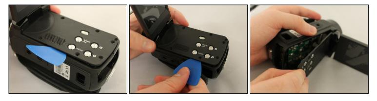
• Use a thin plastic pick to pry off the side of the device and carefully remove the display.
