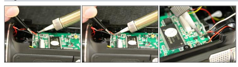
• Use the <u>advanced soldering guide</u> to solder the wire back onto the motherboard.
