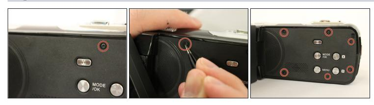
• Use tweezers to carefully pull out the circular stickers to reveal the 4mm screws.
