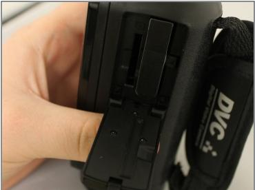
• Pull back the bottom tab to reveal the battery compartment.
