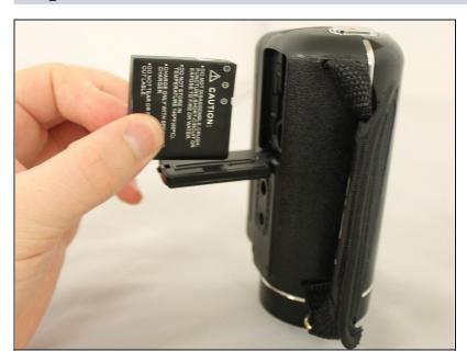
Pull back the tab that is holding in the battery in place and remove the battery from the device.
