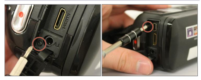
• Use the screwdriver to remove the 2 4mm screws from the port cover.
