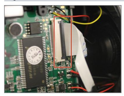
To remove the side face entirely, find the large white connector, flip open the grey lip with tweezers, and gently remove the white connector.
