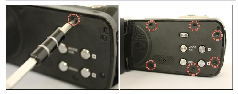
• Use the screwdriver to remove all six 4mm screws from the side of the device.
