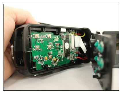
Carefully remove the side face from the device. Avoid pulling on the white connector.
