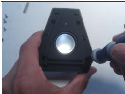
• Take out the four screws, then remove the panel that contains the speaker.
