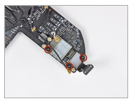
Remove the three 2.6 mm T6 Torx screws securing the AirPort/Bluetooth board to the logic board.
