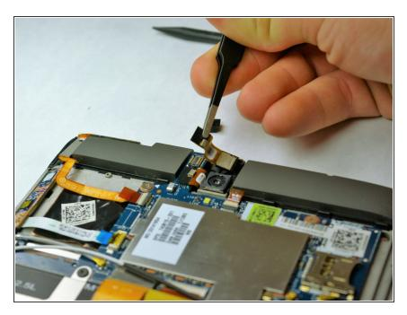
Use ESD safe tweezers to pry the camera away from the motherboard starting at the side opposite the ribbon cable.
