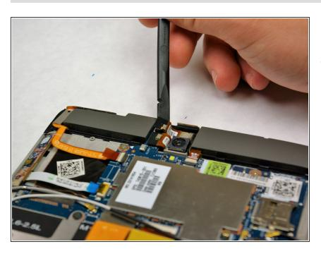
Use the Spudger to disconnect the ribbon cable to the upper camera by prying the connector away from the board.
