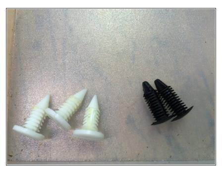
The original retainers (white) and the replacements I found (black). The replacements are AuVeCo #19149: 3/8" head, 7/32" stem width, 5/8" length. Fastenal carries them with SKU 11120582 for a box of 50 (I needed 42).
