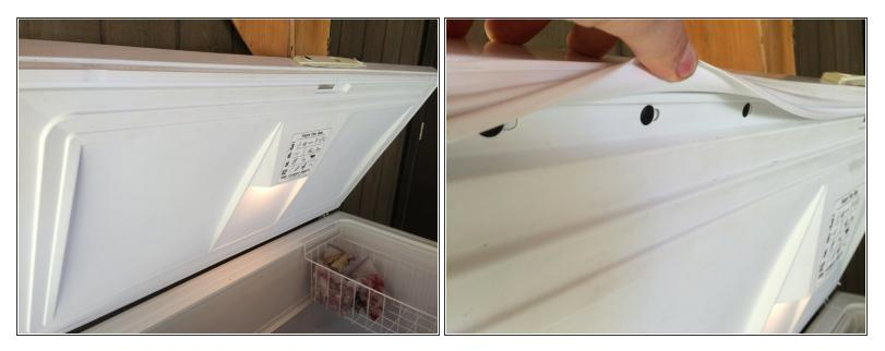
• The lid is a steel frame around a solid foam panel. The inside of the lid is a thin plastic molded cover held on with plastic push-in retainers (under the gasket). The plastic cover is too thin to be able to use metal screws as a replacement.
