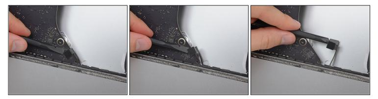
• Use the flat edge of a spudger to pry the headphone jack cable connector from its socket on the logic board.
