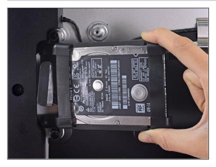
• Remove the hard drive assembly from the iMac.
