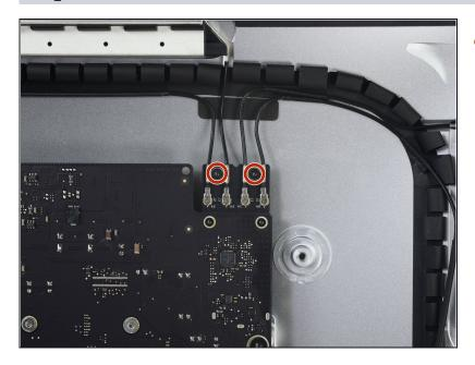
Remove the two 4.0 mm T5 Torx screws securing the four antenna connectors to the AirPort/Bluetooth card.
