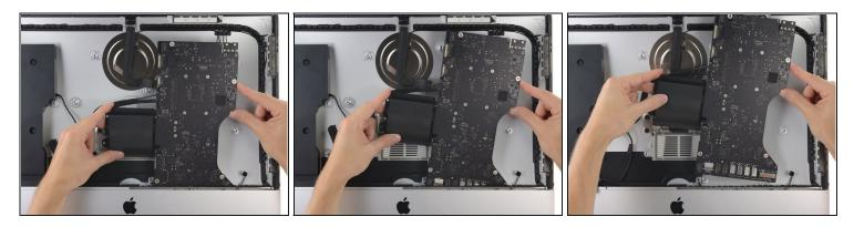
• Lift the logic board straight up and out of the iMac.
