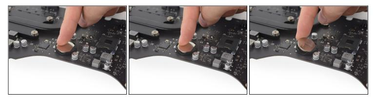
(i) The PRAM battery is secured by a spring contact and two small plastic nubs.
