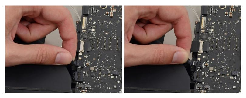
• Gently pull the fan cable connector straight out of its socket on the logic board.
