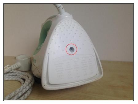
• Remove a Torx security screw from the rear of the iron.
