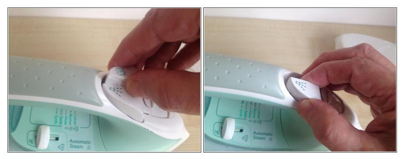
• Remove the two steam buttons. These just pull out. To get the first one out, press the other so you can grip the one you're trying to remove.
